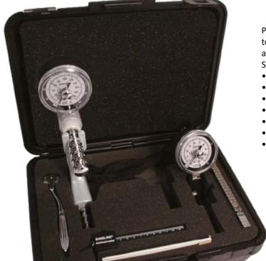
Portable carrying case contains all instruments necessary to evaluate the strength and range-of-motion of the hand
